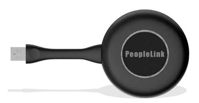
The **Wireless Presenter** is an advanced tool designed to enhance meeting and collaboration experiences by seamlessly connecting room displays with remote participants. The dongle wireless collaboration system allows users to wirelessly integrate cameras, microphones, speakers, and displays with laptops during meetings, offering reverse transmission capabilities for both video and audio.
